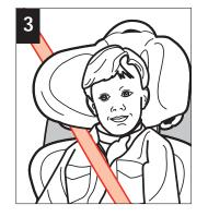
Secure the shoulder belt through the shoulder belt positioning guide in the headrest. The belt should cross the base of the child's neck and across the chest (not the face or neck). Adjust headrest as needed (see "Headrest Adjustment" section). Pull up on the shoulder belt to tighten. Check periodically to ensure your child has not
